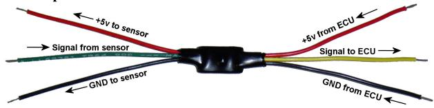
**NOTES:** The two **RED** and the two **BLACK** wires are tied together internally. One pair must be supplied with power, typically available from the same connector as used for the "**Signal to ECU**" connection. The other pair can be used to power the sensor if needed (e.g., a pressure sensor). CUT THE BARE, UNUSED POWER WIRES IF YOU DO NOT NEED THEM! DO NOT LEAVE THEM EXPOSED!
